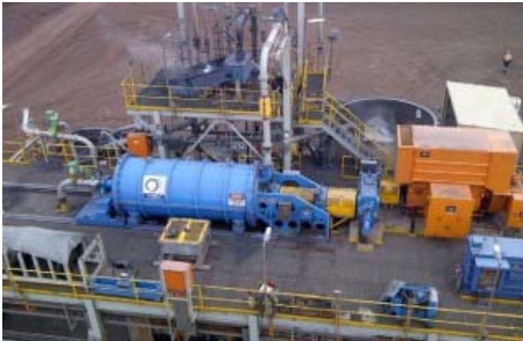
*There is a Glencore Technology M10,000 IsaMill operating at Arrium’s magnetite operation in South Australia*
