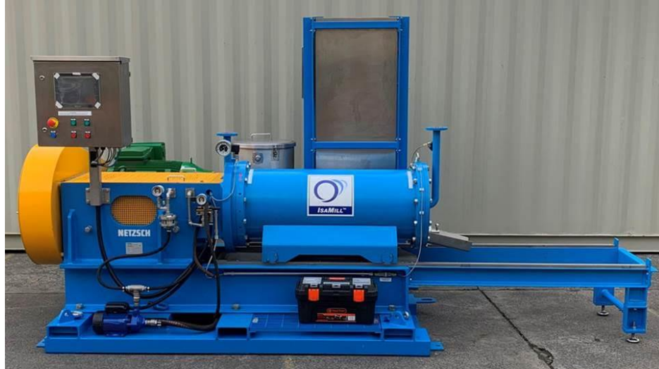
Figure 12: M100 IsaMill™ (Current Coarse Grinding Signature Plot Pilot IsaMill™)
